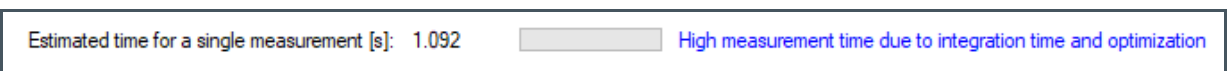
Figure 31: Calculated Measuring Time And Loading Bar In Main Tab If Measuring Time > 1 sec
